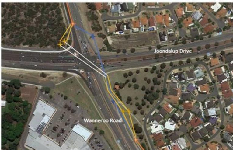
Once Cape Utilities has completed drilling, and new poles are installed, Western Power will remove two steel poles no longer required and the redundant overhead wires that cross the intersection. It is expected these works will be completed in April 2019.
